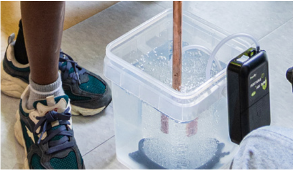
▲ Students demonstrating pile driving with the bubble curtain activated.
